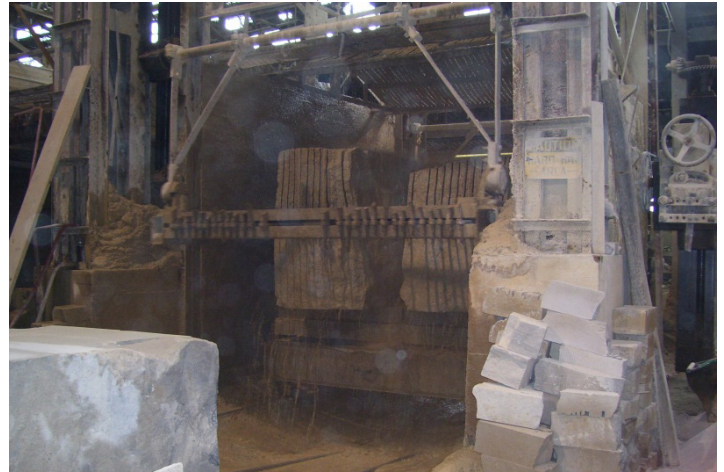
Sawing stone at Bybee Stone Co. ↓
