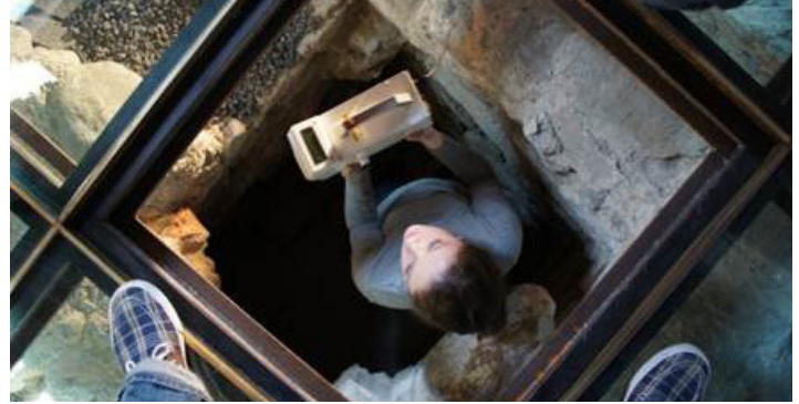
↑ Sarah collecting data in church ruins using a psychrometer (measure temperature and humidity) and fangerometer (measures air velocity).
